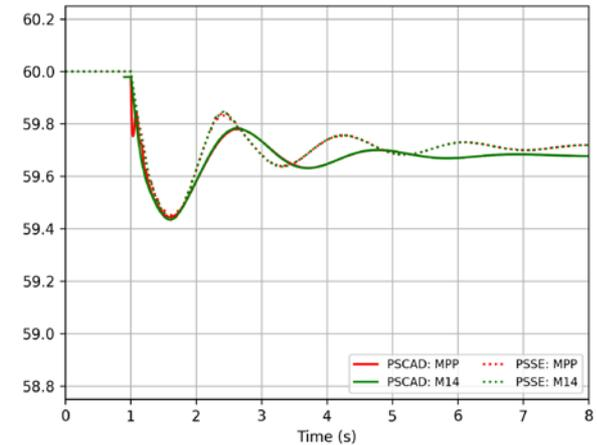
PSCAD: MPP is a PLL-measured frequency. PSCAD: M4 is a generator shaft rotation speed derived frequency
