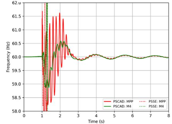
PSCAD: MPP is a PLL-measured frequency. PSCAD: M4 is a generator shaft rotation speed-derived frequency
