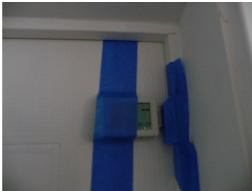
Figure A8. Door open/close sensor on IZ door
