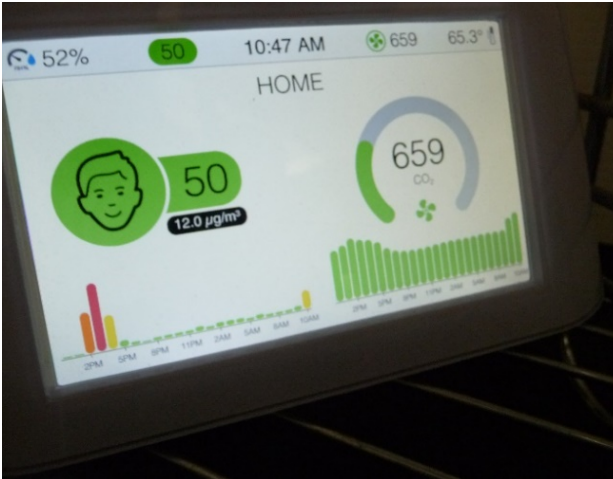
Figure A6. Screen of the Air Visual Pro PM 2.5 sensor used in study
