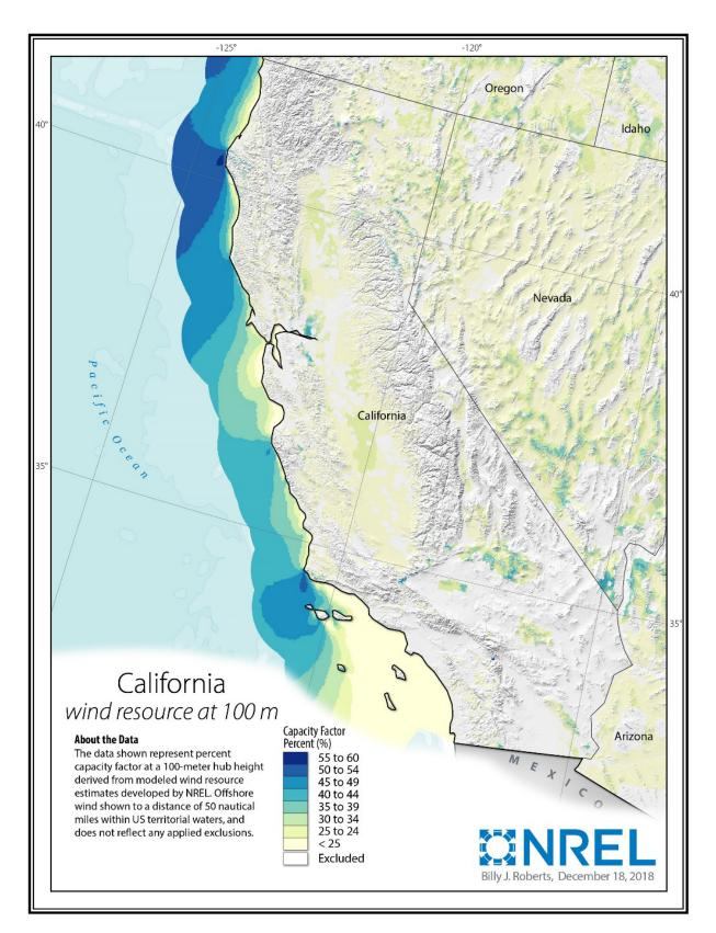
Figure 23. Capacity factor for potential wind sites in California, with land exclusions applied
