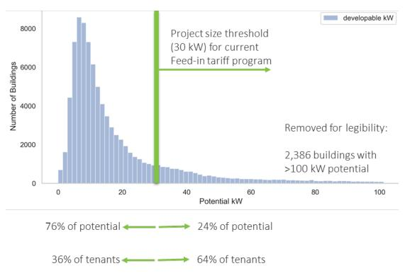
Figure 11. Histogram of rooftop solar potential for multifamily buildings with technical potentials >100 kW
