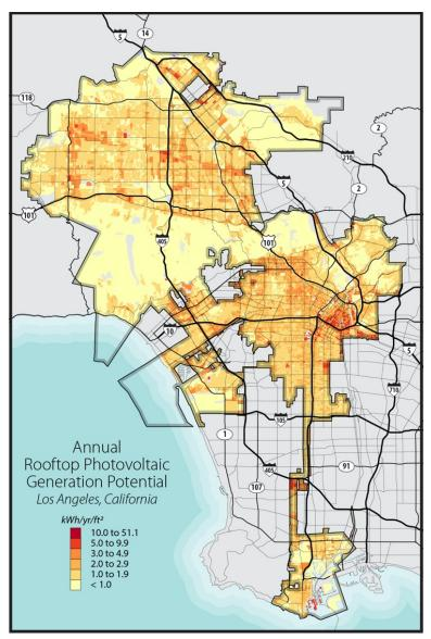
Figure 10. Annual rooftop solar PV generation potential (kWh/yr/ft<sup>2</sup>) in 2019 based on lidar scans, averaged by census tract
