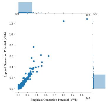
Figure 27. Scatter plot of empirical rooftop generation potential (x-axis) to imputed value (y-axis)
