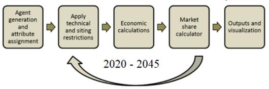
Figure 6. Flow diagram for dGen model
