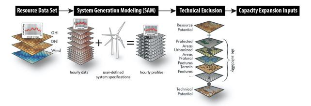
Figure 22. Process flow of the Renewable Energy Potential (reV) model
