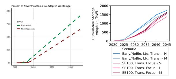
Figure 21. Projected distributed storage co-adoption rates (left) and deployment (right)
