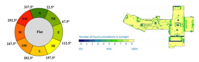
Figure 26. Categorization of roof plane orientations (left) and visualization of roof plane irradiance based on plane tilt, azimuth, and shading (right)
