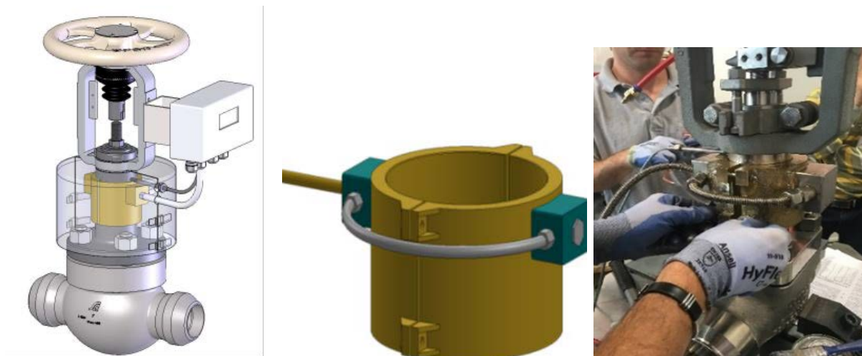
Figure 40. Valve self-contained thermal management system
