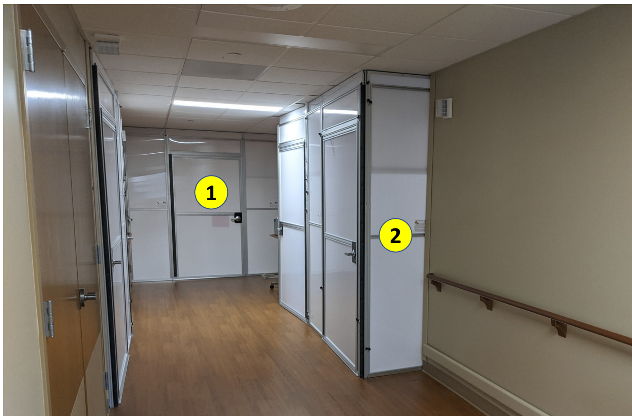
Figure 1. Experimental isolation test space (1 = controlled entrance, 2 = temporary anterooms)
