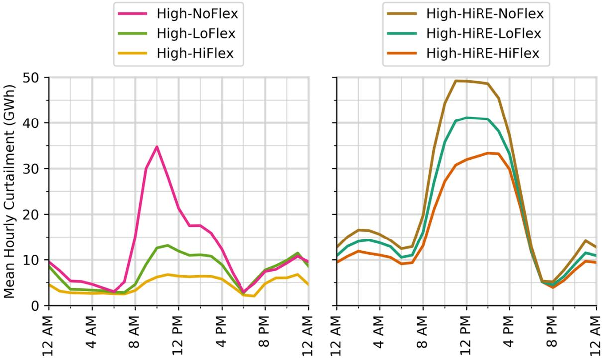
Figure 29. Mean hourly renewable curtailment in High-No/Lo/HiFlex scenarios (left) and High-HiRE-No/Lo/HiFlex scenarios (right)
