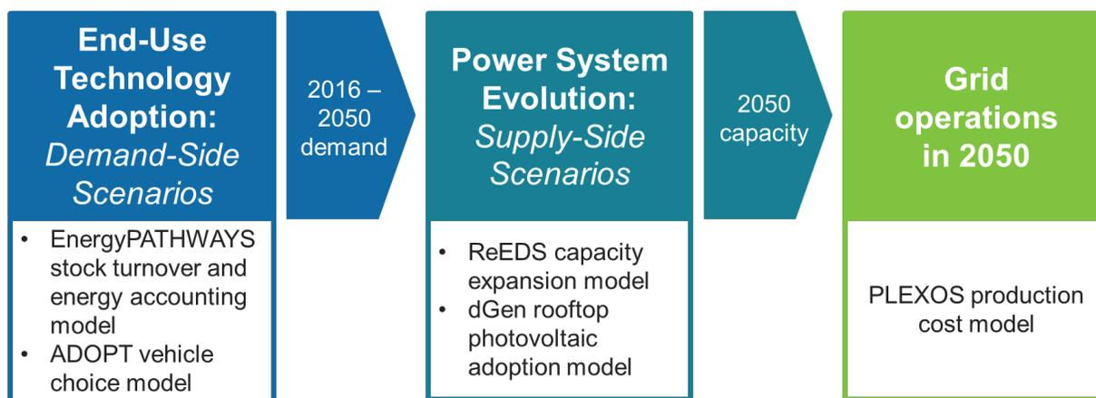
Figure 1. Electrification Futures Study structure and scenario analysis
