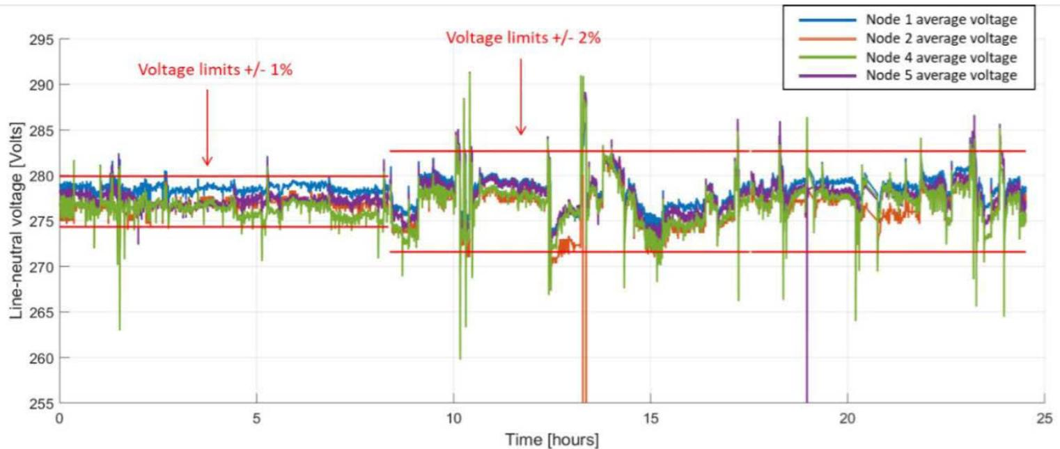
Figure 11. Average line-neutral voltage at nodes in the microgrid
