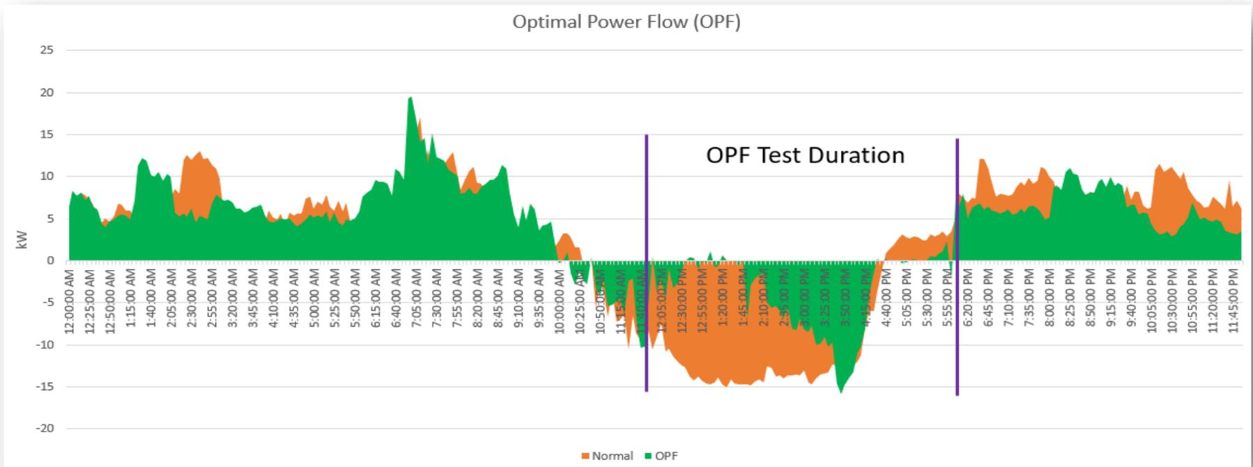
Power at Transformer set to 0 Watts throughout. System set to aggregated optimization. PV set to charge batteries than to grid. Option to curtail PV to create a true 0 Watts load profile.
