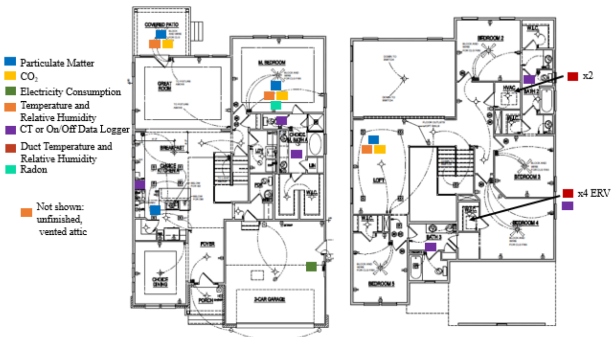
Figure 10. IAQ sensor and ventilation performance sensor location map (typical), 1st floor (left), and 2nd floor (right)
