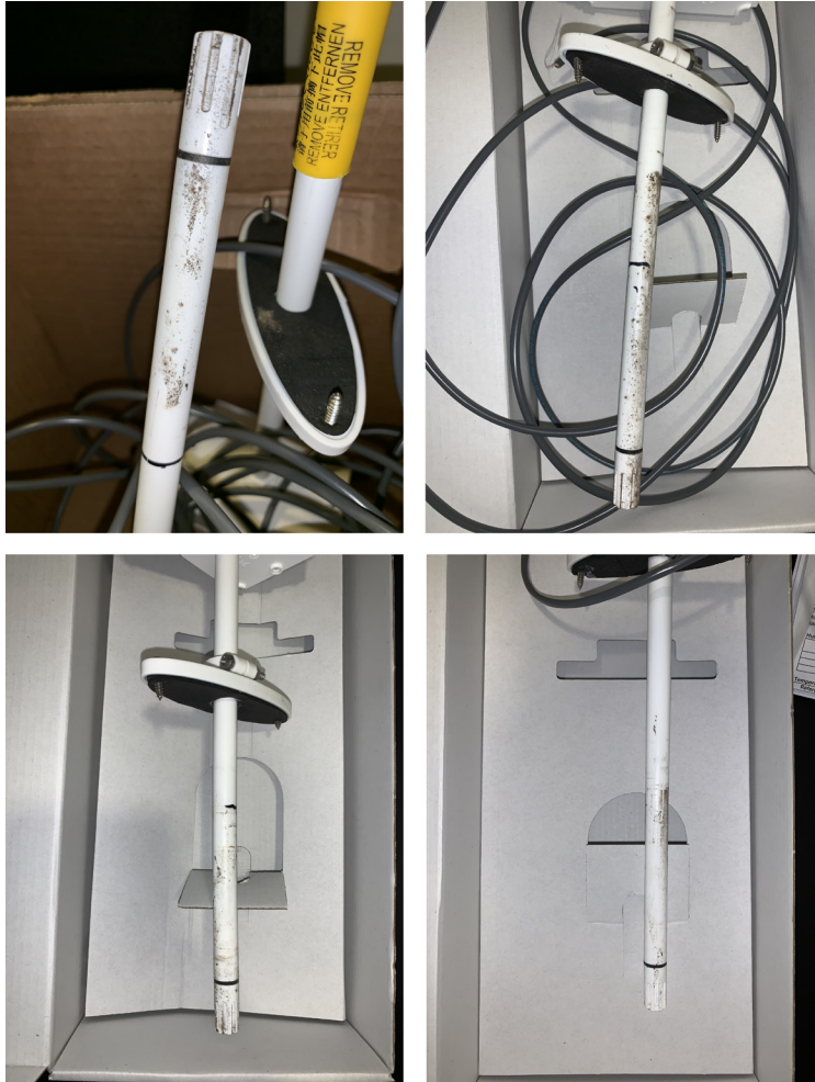
Figure 26. Photos of each of the X_1 duct probes from test homes 1–4 (clockwise, from top left)
