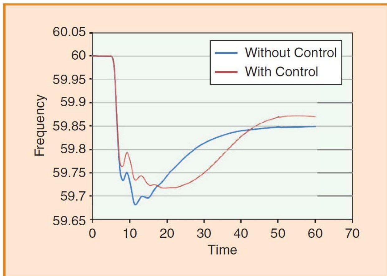
Figure 3- 4. VRE with and without synthetic inertia controls
