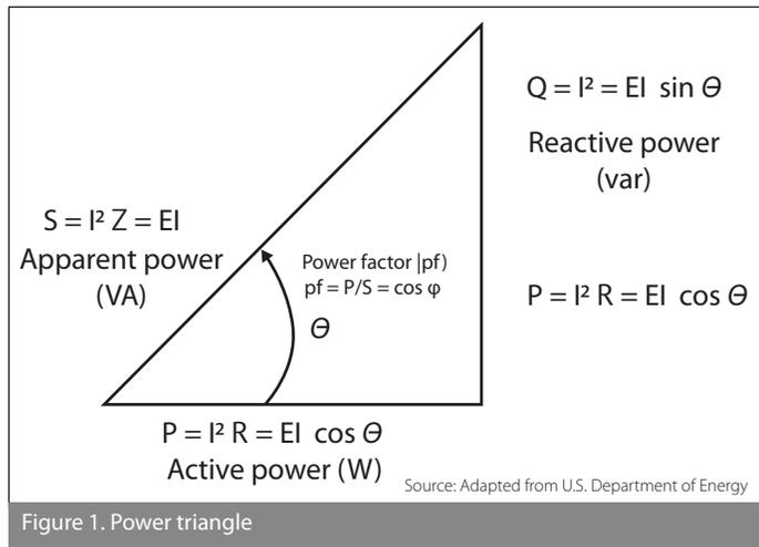
The equations for calculating these values from basic electrical quantities of root mean square voltage (E), resistance (R), reactance (X), impedance (Z), and root mean square current (I) are also shown in Figure 1.
