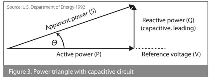
Typical distribution circuits contain resistive and inductive loads; therefore, utilities install capacitors to balance the var requirement (Blume 2007).
