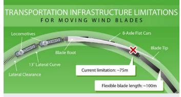
High-energy-capture machines with highly flexible blades open many more parts of the United States to wind development by solving logistical and science challenges associated with these machines.
