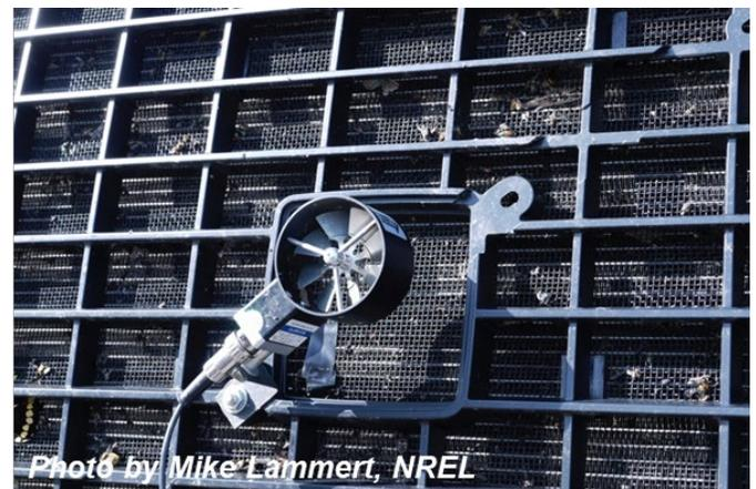
Figure 7. Photograph of anemometer mounted on the center of grill
