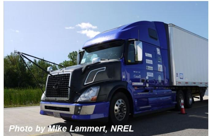
Figure 2. Photograph of boom for mounting boom location probe and thermocouple ahead of vehicle hood
