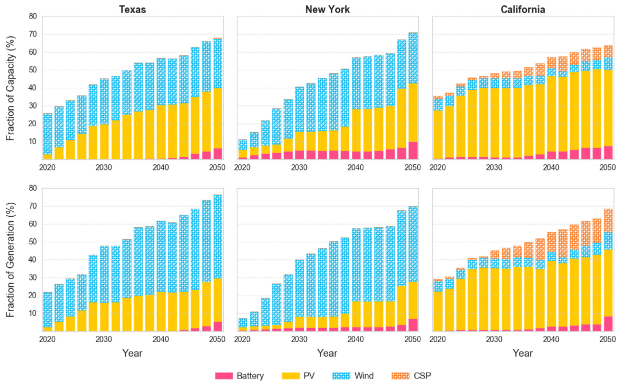
Fig. 2. Capacity fraction (top) and generation fraction (bottom) of battery, PV, wind, and CSP in each region.
