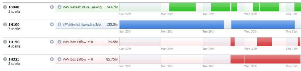
Figure 3. Zone-level fault detection and diagnostics
