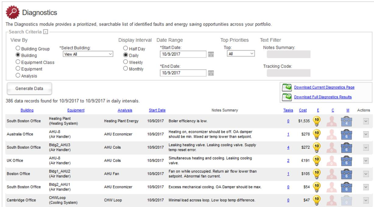
Figure 4. A prioritized list of faults detected
