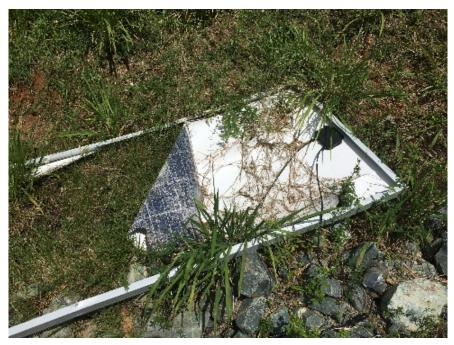
Figure 33. PV module torn from racking, lying facedown, shows laminate failure. *Photo by Eliza Hotchkiss, NREL*
