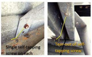
Source: Robinson, Walker, and Fu (2018) Figure 35. Examples of hardware failure
