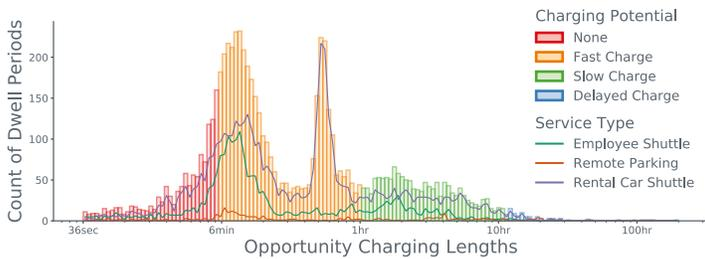
Idle times for existing shuttle routes demonstrate opportunities for on-route and between-service electric vehicle charging. Figure by Andrew Kotz, NREL
