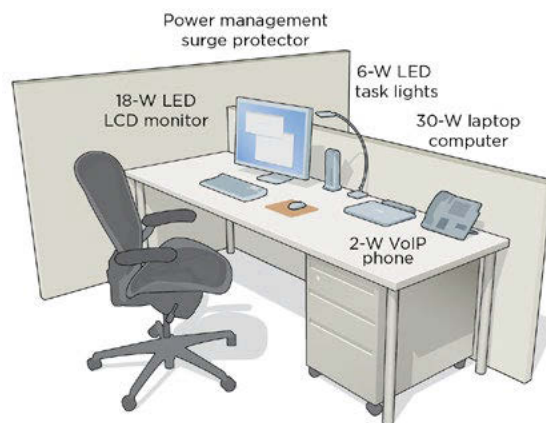
Figure 7. Diagram of an example low-energy workstation. Illustration by Matthew Luckwitz, NREL
