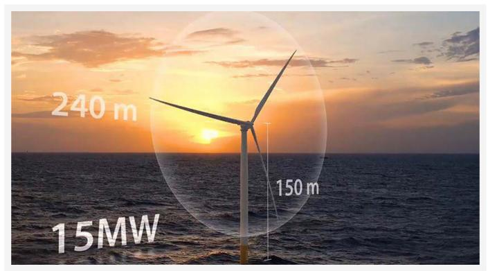
An artistic rendering of the IEA Wind 15-MW Reference Turbine. The open-source offshore turbine design allows wind industry contributors to share their designs and innovations with other researchers to accelerate technological development. *Illustration by Josh Bauer, NREL Photo by Werner Slocum, NREL*
