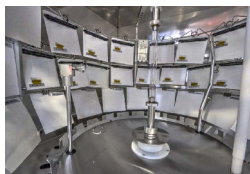
MiMo and coupon specimens in Xe Ci5000 chamber for IEC 62788-7-2 method A3 weathering.
