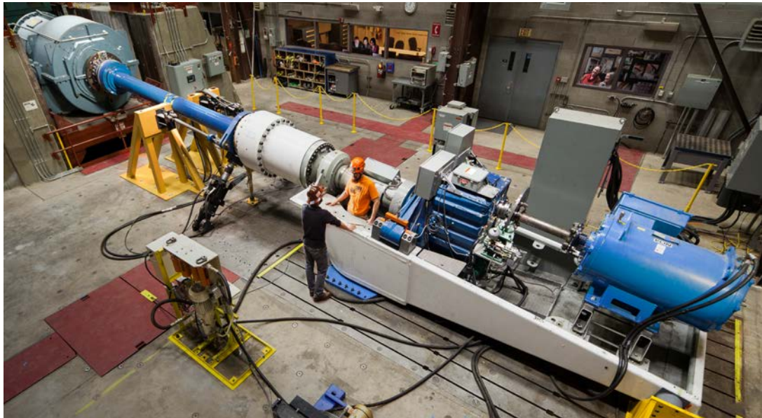
Figure 3 – Dynamometer experiment setup of 750-kW wind turbine drivetrain. Photo by Mark McDade, NREL 32734
