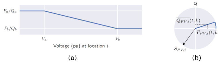
Figure 6. (a) Piecewise linear VW/VVAR droop curve. (b) Maximum reactive power for VVAR is limited by power factor and inverter rating.
