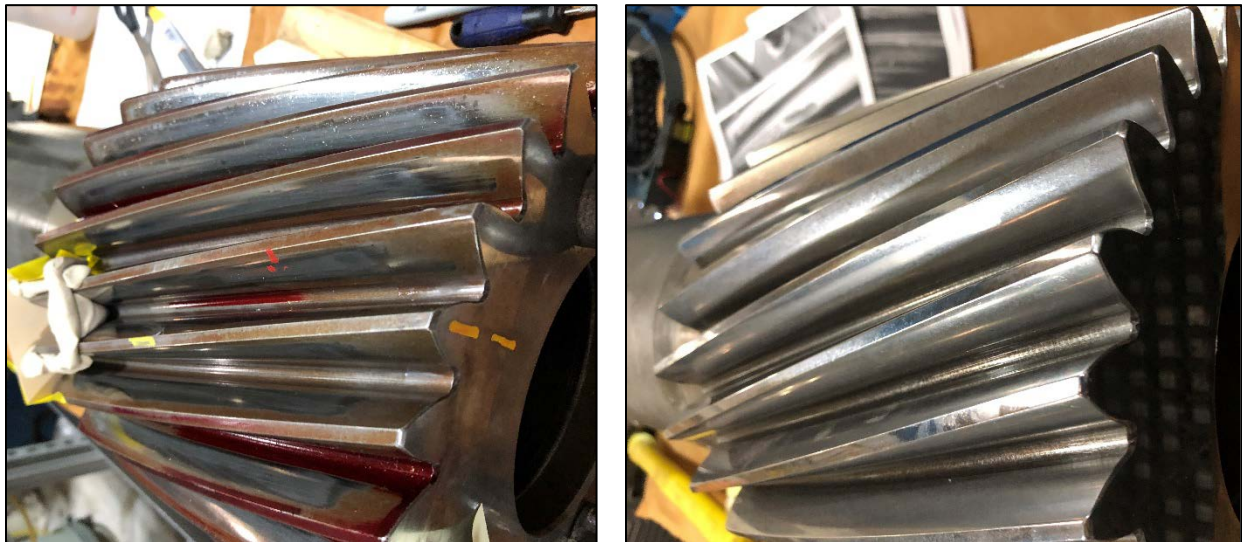
Figure 8. Sun pinion before (left) and after (right) isotropic superfinishing
