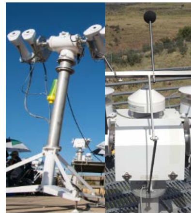
Fig. 2. NREL's BORCAL method, which involves a self-calibrating, absolute cavity radiometer (left) and a diffuse pyranometer on a tracker (right). Photos by NREL
