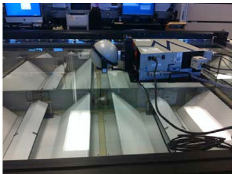
Fig. 3. NREL’s spectroradiometer calibration setup traceable to the National Institute of Standards and Technology: a tungsten-filament, 1,000-W quartz-halogen FEL (top), and a spectroradiometer (bottom) are used to calibrate a solar simulator. Photos by NREL
