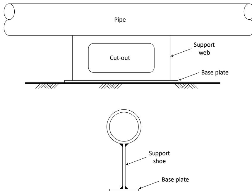
**Figure 6-10. Candidate metal pipe support**
