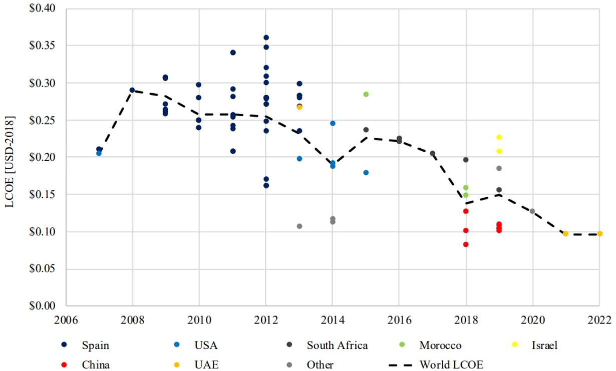
**Figure 1-1. Levelized cost of electricity (LCOE) of the 77 solar-only commercial CSP stations for which csp.guru has data on both cost and expected generation for 2006–2018 (operational) and 2019–2022 (under construction in January 2019, scheduled completion 2019–2022). The average LCOE is the generation weighted average of all stations (expected) to start operating in each year.**
