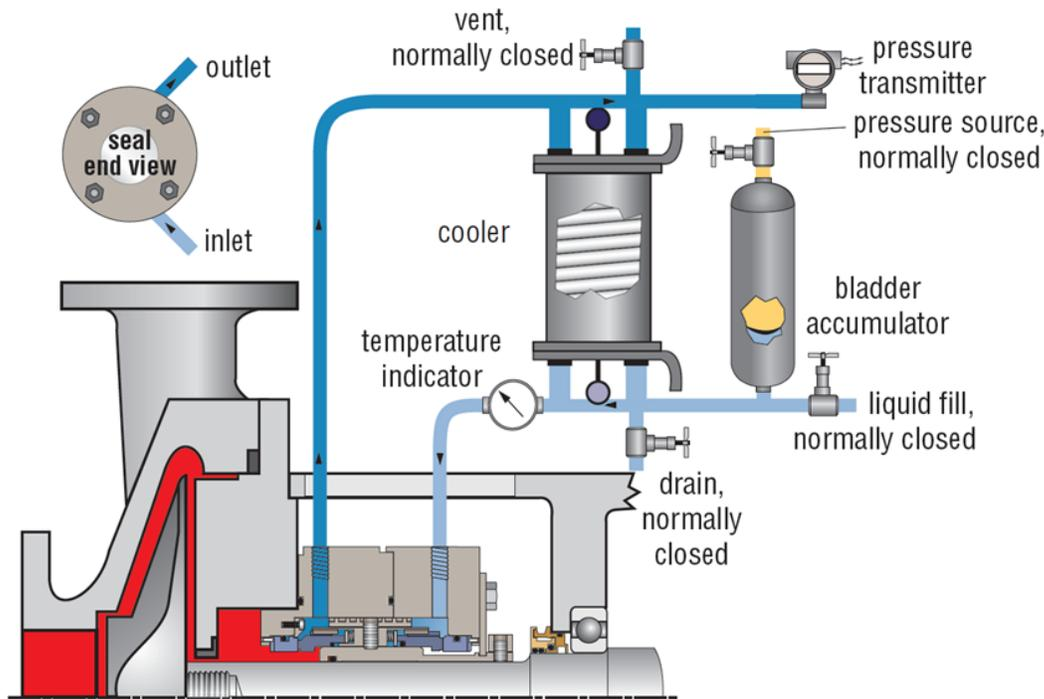
**Figure 5-4. Common piping plan, 53B**
