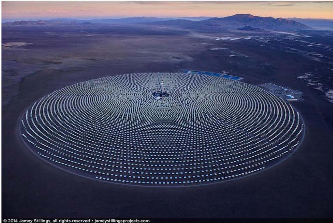
**Figure 6-4. Crescent Dunes heliostat-field layout for salt receiver**
