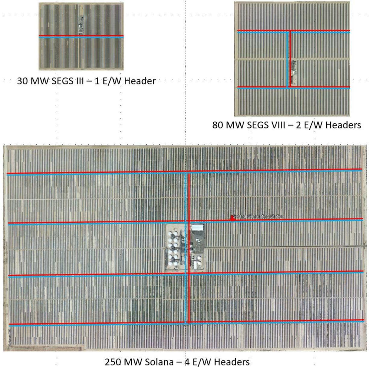
**Figure 5-2. Ideal rectangular layouts for solar field with for 1, 2, and 4 headers**
