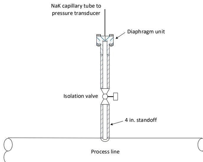
Figure 6-9. Diaphragm pressure transmitter on 4 in. standoff
