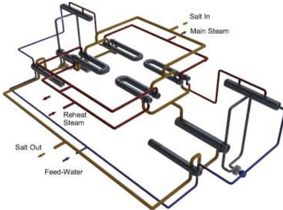
**Figure 6-6. Steam-generator arrangement with two 50% trains**
