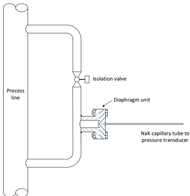
**Figure 6-11. Pressure-transmitter installation**
