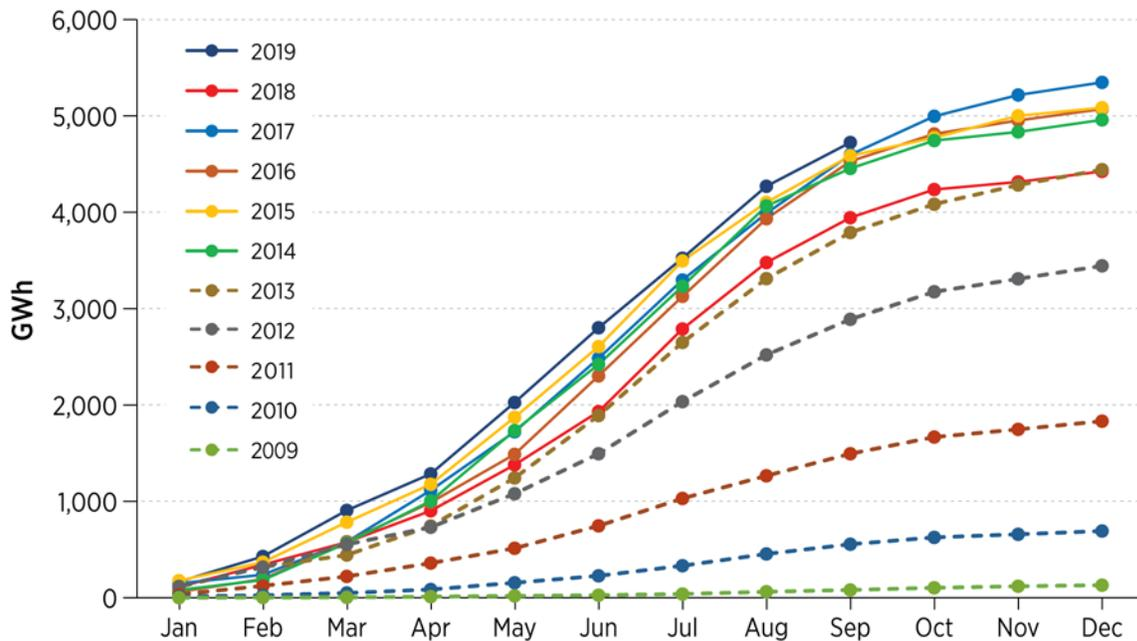
**Figure 1-2. Monthly cumulative generation of Spanish CSP plants (Protermosolar). Dashed lines represent continued construction of CSP plants. Solid lines represent increased output from plants considering no additional construction. Reduced performance in 2018 is due to a significant reduction in direct normal insolation in Spain that year (Protermosolar).<sup>2</sup>**
