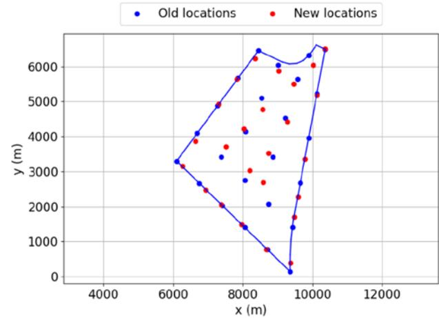
$$\underset{x,y,\gamma}{\text{minimize}} \quad - \sum_{i=1}^{N_{turb}} P_i(x_i, y_i, \gamma_i, w_s, w_d, f)$$
