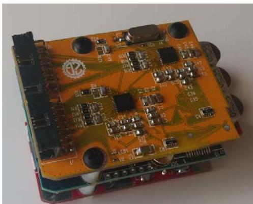
Figure 35. Representative submeter circuit board
