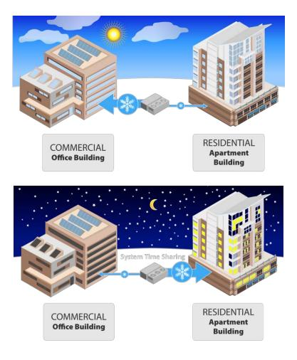
Figure 8: Some CCs Take Advantage of Load Diversity to Minimize CAPEX Credit: NREL-Marj Schott
