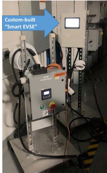
Figure 5. ANL's custom-built EVSE with cloud-based controls
