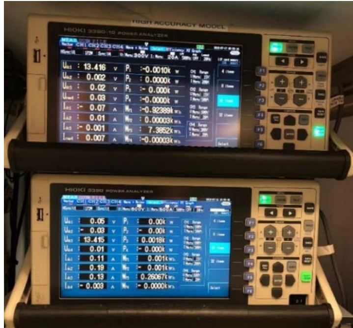
Figure 6. Hioki 3390 Power Analyzer meters (four channels each). The main display shows the values of voltages, current, and power of the selected nodes. The data is logged and saved in csv format, which is then merged with the vehicle CAN data.
