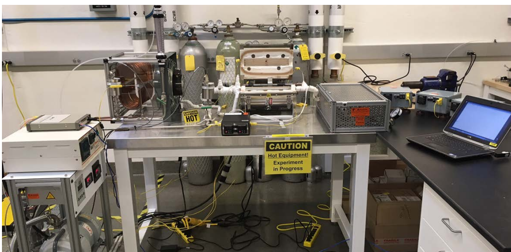
Figure 45. Laboratory test layout for testing the integrated hydrogen sensor and separation module.
