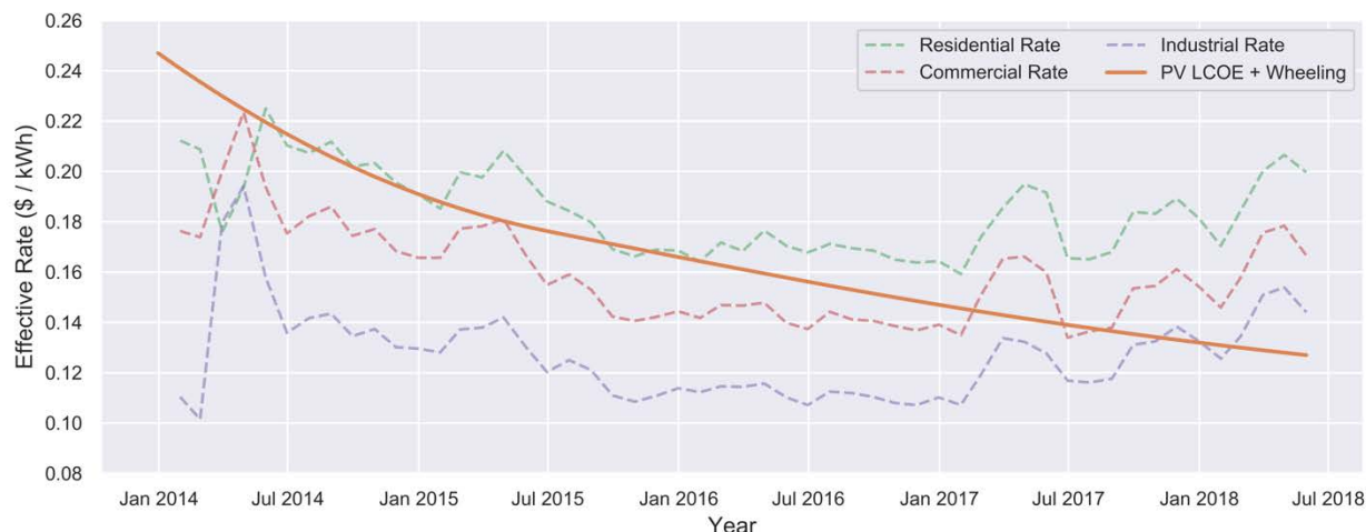
Figure 4. Historic MERALCO rates compared with solar levelized cost of energy + wheeling charges
