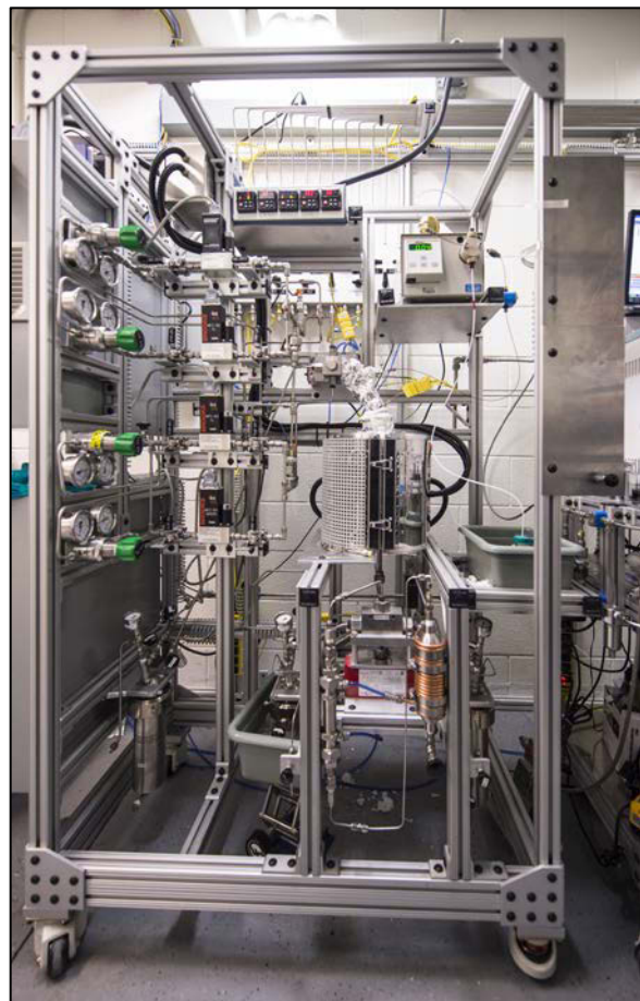
C3PO: a high-pressure trickle bed flow reactor
