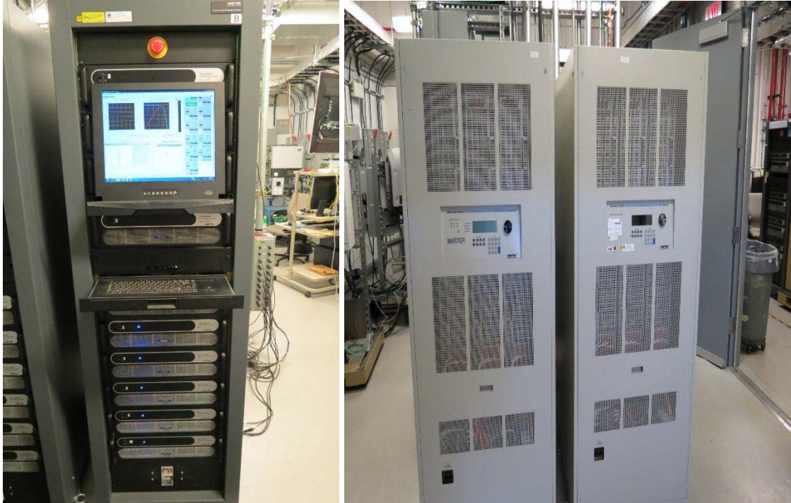
Figure 3. Lab equipment at Sandia for evaluating conformance test procedures: TerraSAS100-kW PV simulator (left); Ametek 180-kVA AC simulator (right). Photos courtesy of Sandia National Laboratories
