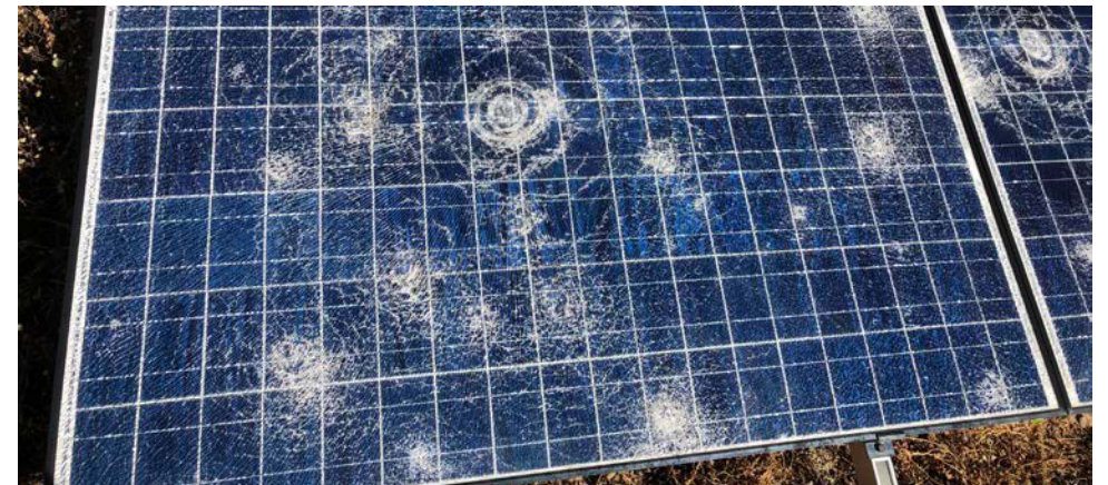
PV panels damaged by hailstorm. Photo by Andy Walker
