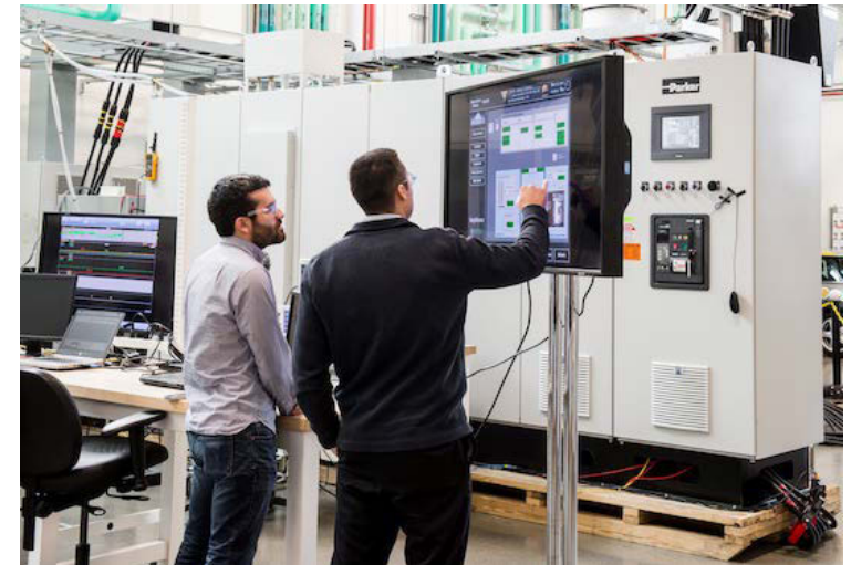
NREL and Raytheon, perform system level testing on the Miramar ZnBr Flow Battery Photo by Dennis Schroeder / NREL 32582
