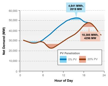
Figure 4: Change in California net load shape due to PV. Adapted from Denholm and Margolis (2018)
