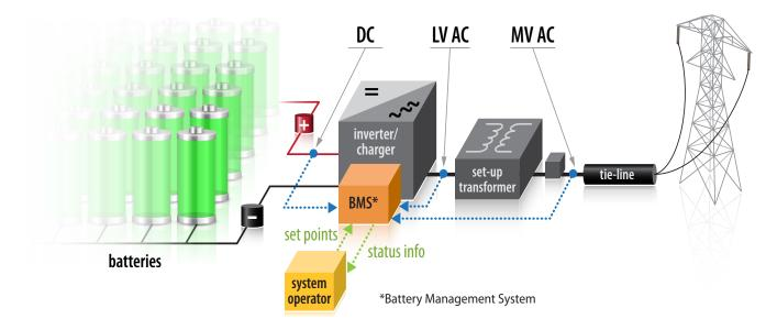
Figure 3: Key components of BESS interconnected at the transmission substation level. LV AC represents a low-voltage AC connection, while MV AC represents a medium-voltage AC connection.<sup>4</sup> Source: Denholm (2019)
