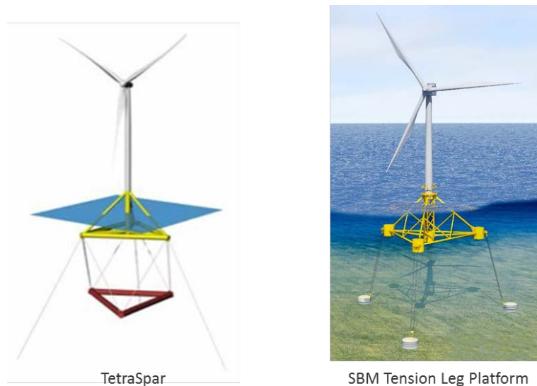
Figure 31. Second-generation floating wind concepts of alternative hybrid substructures. Images courtesy of Stiesdal Offshore Technologies (left) and SBM Offshore (right)
