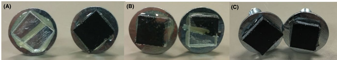
FIGURE 6 Examples of different failure modes. A, 100% adhesive failure. B, ~70% adhesive ~30% cohesive failure. C, 100% cohesive failure
