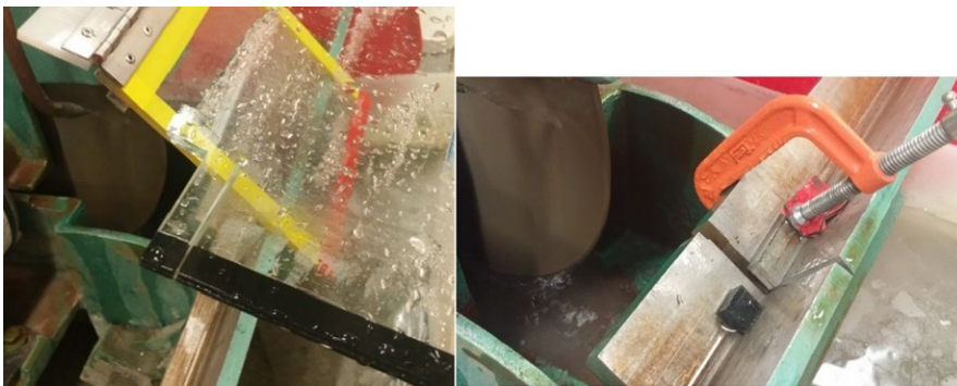
FIGURE 2 Photos showing specimen removal using a tile saw
