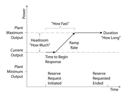
Figure 5. The three characteristics of operating reserves.
