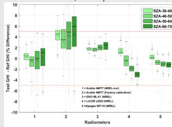
Fig. 3. Irradiance comparison of photodiode sensors relative to the reference data (1-min data set from 8/18/2017 to 11/28/2017)
