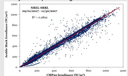
Fig. 4. One-minute GHI comparison between Arable Mark and a reference CMP22 thermopile pyranometer
