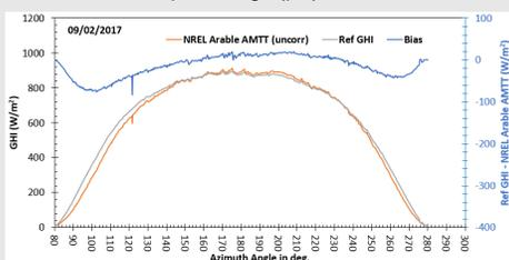
Fig. 2. Measured irradiance from the reference data set and the UUT as well as directional bias. The data from 09/02/2017 are used to calibrate the UUT using Eq. 1.
