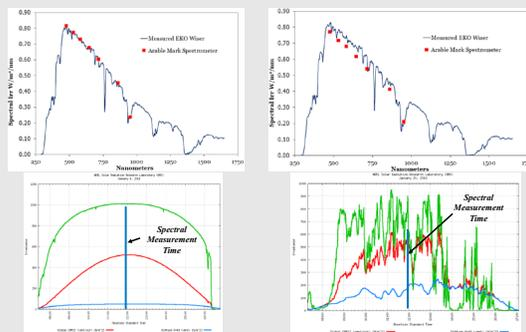
Fig. 5. (Top) Spectral comparison between the WISER and Arable Mark for 01/04/2018 @ 12:00 LST; (bottom) broadband direct (green), global (red), and diffuse (blue) irradiance measured with thermopile radiometers for that clear day (left) and the same but for partly cloudy skies for 01/20/2018 @ 12:00 LST (right)
