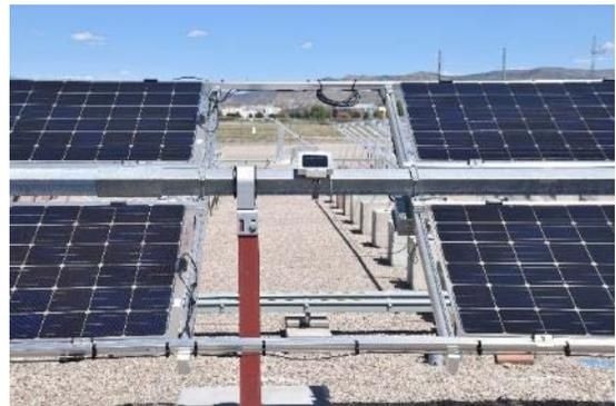
Fig. 2. Sandia bifacial tracking array with front and rear irradiance sensor shown (center). Two rows with GCR 0.28
