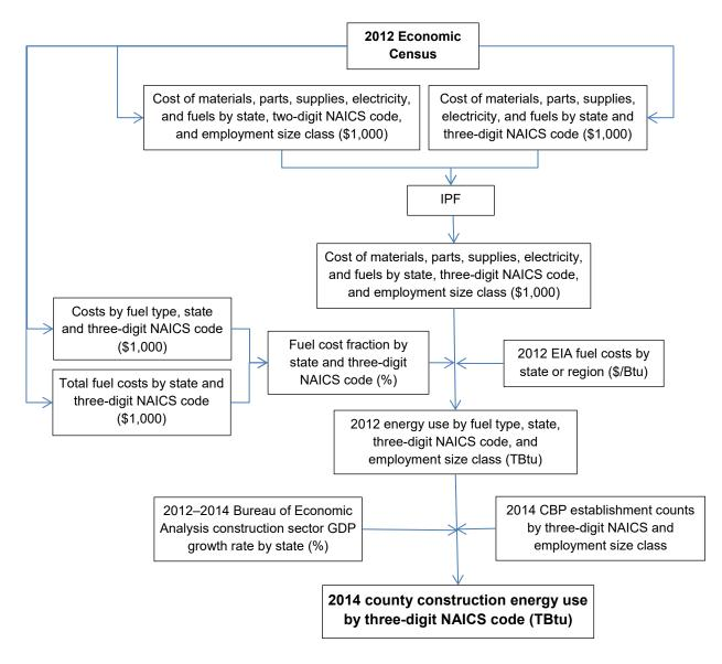
Figure 3. Overview of county-level construction energy calculation
