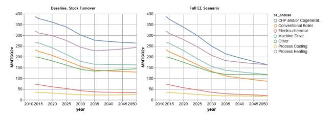
Figure 16. IET baseline and energy efficiency scenario projected emissions by end use CHP = combined heat and power, EE = energy efficiency, MMTCO2e = million metric tons of carbon dioxide equivalent, and ST enduse = energy end use category
