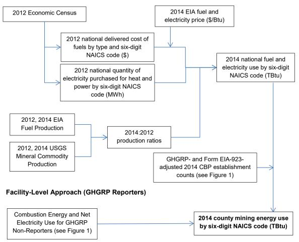
Figure 4. Overview of county-level mining energy calculation
