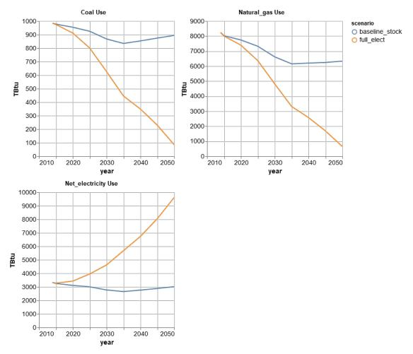
Figure 13. IET national projected coal, natural gas, and electricity use in baseline and fuel switching scenarios
