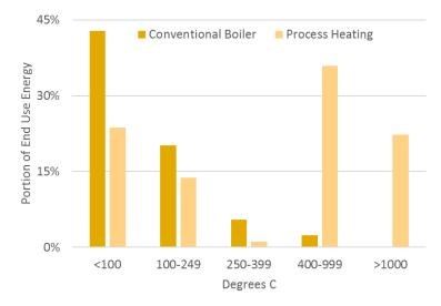
Figure 5. Associated temperature range for 2014 county-level conventional boiler use and process heating energy use
