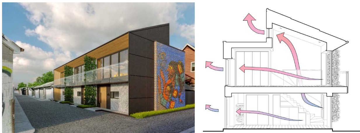
Figure 4. (a) LaneZero and (b) diagram of the LaneZero natural ventilation (Ryerson University, University of Toronto 2017)
