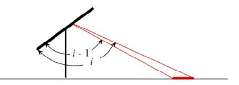
• Diffuse irradiance for back-side is summed by dividing field-of-view into 180 onedegree segments and adding each segments contribution
