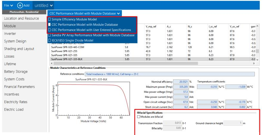
• Bifacial model available for module models which do not require test data
