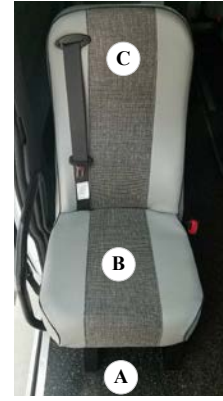
Fig. 8: Test points for the driver's seat inside the bus.
