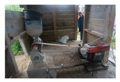
Figure 10: Diesel powered milling machine
