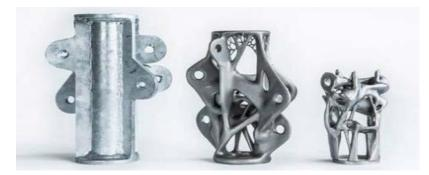
Figure 16. Arup steel structural member in original form (left) and AM (center and right) (Protocam 2017). Photo credit: Davidfotografie.
