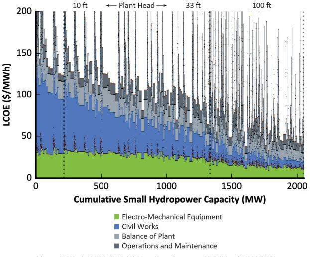
Figure 12. Modeled LCOE for NPD projects between 100 MW and 2,000 MW
