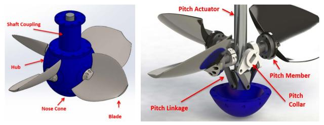
Figure 8. NREL CAD model of the components from the manufacturing analysis
