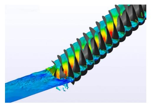
Figure 17. Stress distribution on a composite Archimedes screw turbine (Straalsund 2017) Photo credit: Image courtesy of Pacific Northwest National Laboratory.
