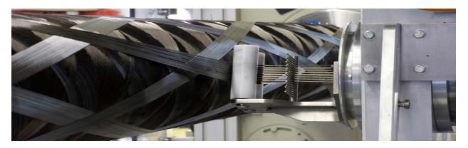
Figure 14. Rotary CF filament winding around a symetrical object (Connova AG 2017). Photo credit: Connova AG.
