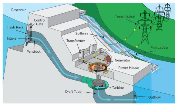
Figure 5. 3D cross-section of a representative hydropower plant and the major components (DOE 2016)
