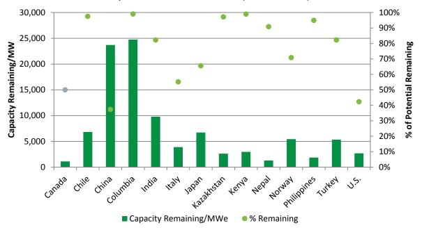
Figure 3. Technical potential of the capacity of SHP remaining by country (MW) and the percentage of the resource still remaining (UNIDO 2016a)
