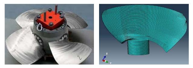
Figure 18. Original runner (left) and wire mesh of composite blade for new runner (Hipp 2017) Photo credit: Composite Technology Development (CTD).
