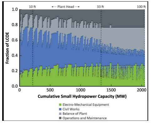
Figure 13. Fraction of LCOE and breakdown of the LCOE for NPDs between 100 MW and 2,000 MW Projects are sorted from lowest to highest head.
