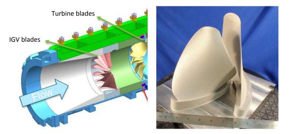
Figure 19. Design of modular section showing the IGV and turbine sections (left) and ½ scale turbine blades produced via metal AM (right) (Fontaine et al. 2017) Photo credit: Arnold Fontaine/Penn State.
