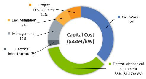
Figure 10. Capital cost breakdown (\$/kW) of a potential NPD site using the representative 2x5 MW turbines
