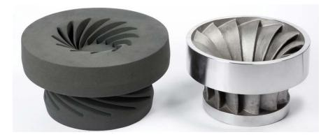
Figure 21. Sand cast made via AM [left] and the resulting runner [right, (Voxeljet AG 2015)] Photo credit: Voxeljet & Wolfensberger.
