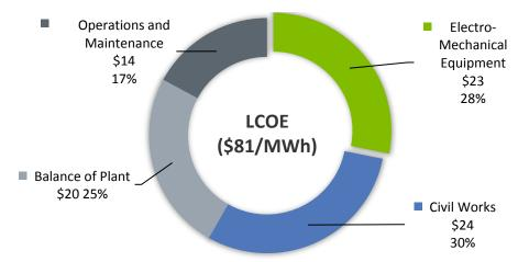
Figure 11. LCOE breakdown for prototypical NPD plant with the 2x5 MW representative turbines
