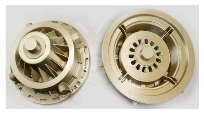
Figure 20. Aluminum gearbox parts produced using 3D-printed sand casts (Shoemaker 2017) Photo credit: Brittany Cramer/Oak Ridge National Laboratory, U.S. Dept. of Energy.
