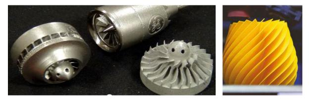
Figure 15. General Electric printed metal turbine representations [left (GE 2013)] and polymer printed part [right (Müller and Karevska 2016)]. Photo credit left: GE Global Research Center. Photo right: iStock 67120779.
