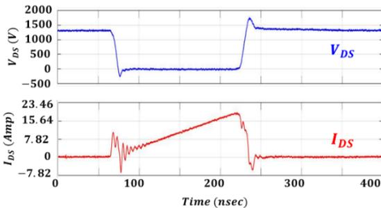
Fig. 7  $V_{DS}$  (top) and  $I_{DS}$  (bottom) waveforms from Switching Cycling as explain in [10].
