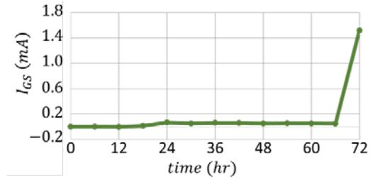
Fig. 9 Changes in Gate-Source leakage over time as a result of Switching Cycling.
