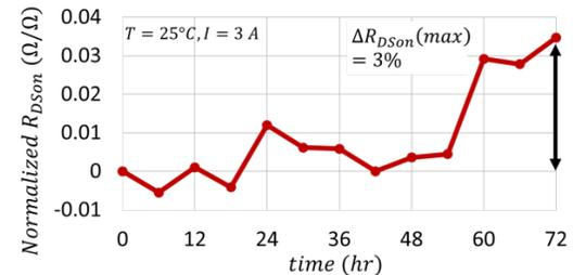
Fig. 11 Normalized  $R_{Dson}$  changes over time as a result of Switching Cycling.
