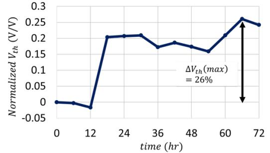
Fig. 10 Normalized  $V_{th}$  changes over time as a result of Switching Cycling.
