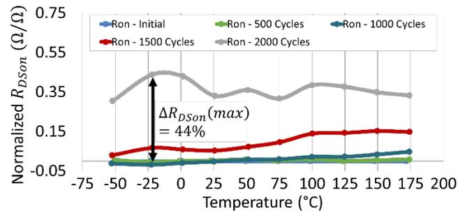
Fig. 16 Normalized changes of  $R_{DSon}$  over time from Thermal Cycling [10].
