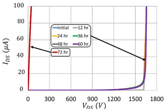
Fig. 8 Changes in Drain-Source leakage current over time as a result of Switching Cycling.
