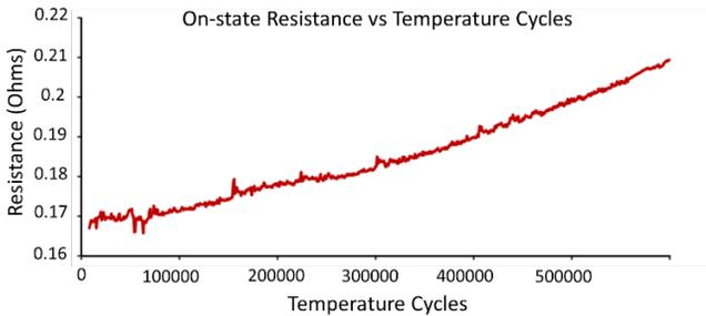
Fig. 13 On-resistance evolution through accelerated test in [15].
