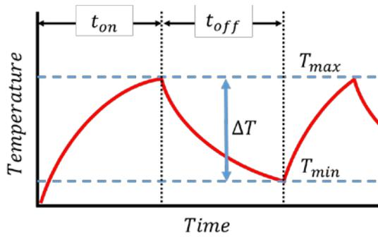
Fig. 12 General temperature stress profile for Power Cycling.
