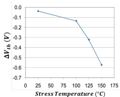
Fig. 6 Dependence of  $V_{th}$  shift on stress temperature for devices with  $V_{GS} = 15$  V,  $t = 1$  hour [8].
