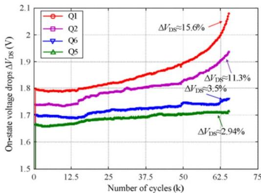
Fig. 14 Measured on-state voltage drop and fitting curves for devices during power cycling tests in [24].
