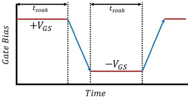
Fig. 2 HTGB experiment showing the soak times for both a  $+V_{GS}$  and  $-V_{GS}$  bias, with ramping voltages between the two bias values [6].
