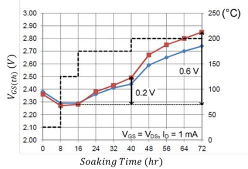
Fig. 3 Static  $V_{th}$  measurements after HTGB tests in [7].
