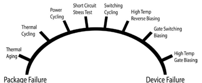
Fig. 1 Accelerated lifetime test spectrum.
