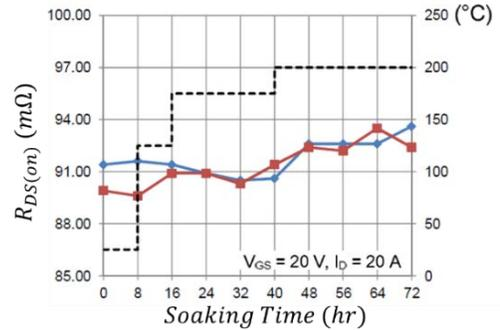
Fig. 4 Static  $R_{DS(on)}$  measurements after HTGB tests in [7].
