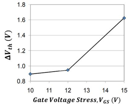
Fig. 5 Dependence of  $V_{th}$  shifts on stress bias for devices with  $T = 150^\circ\text{C}$  and  $t = 1$  hour [8].
