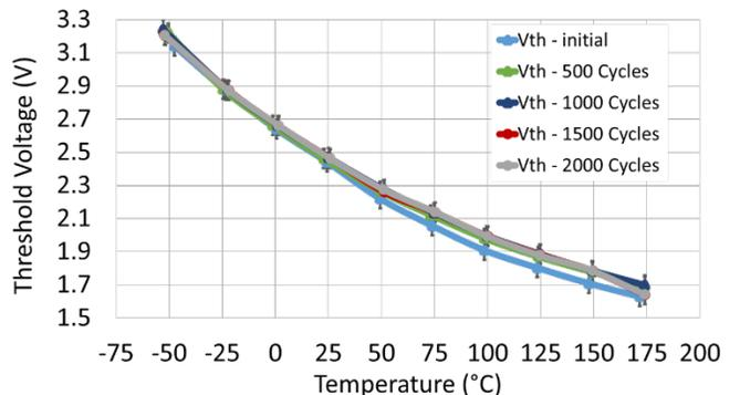
Fig. 17 Changes in  $V_{th}$  over time from Thermal Cycling [10].
