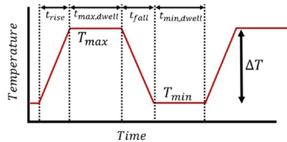
Fig. 15 General Thermal Cycling temperature profile.
