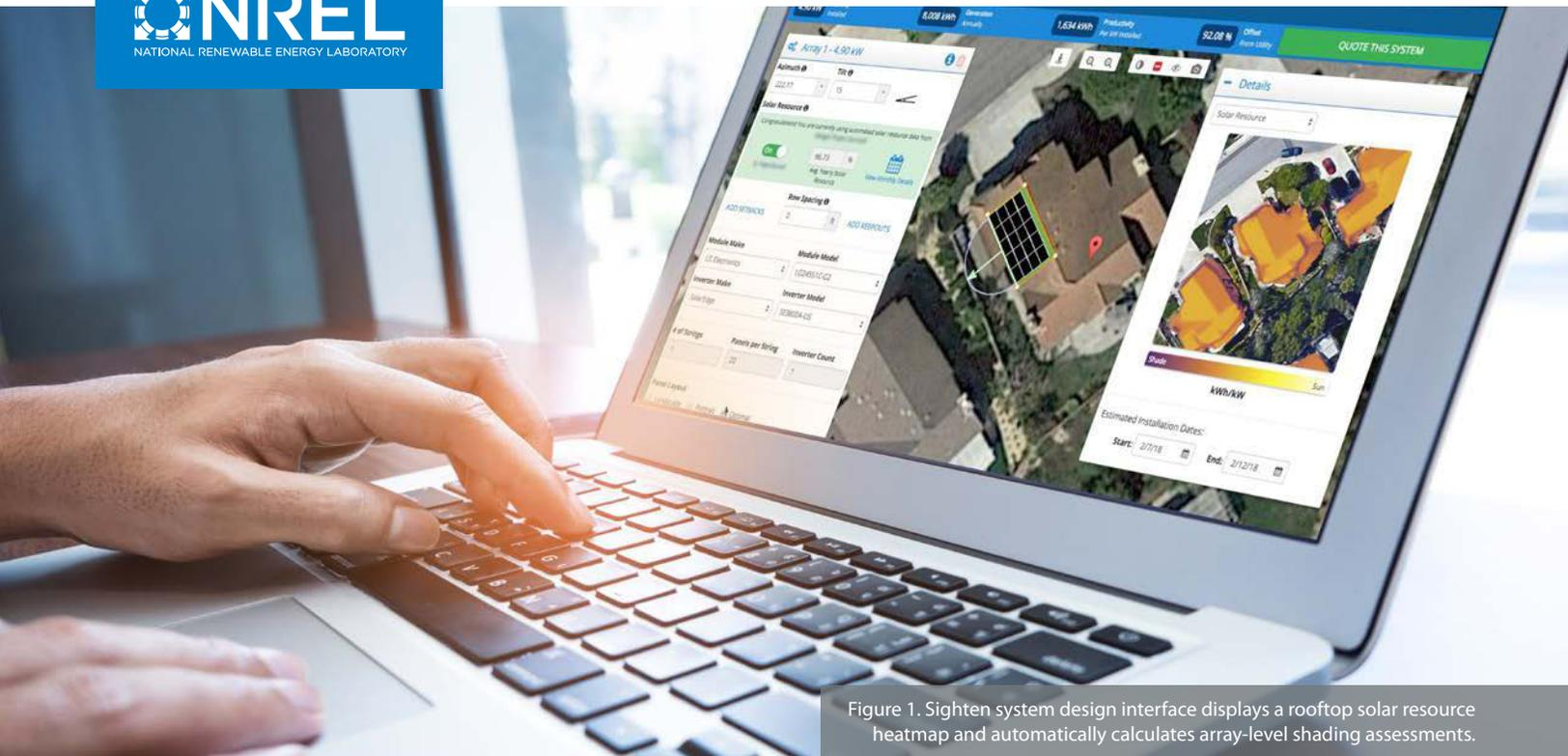
Figure 1. Sighthen system design interface displays a rooftop solar resource heatmap and automatically calculates array-level shading assessments.
