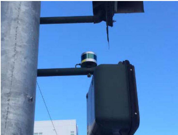
LiDAR sensor mounted at an intersection
