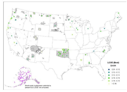
Figure 21. Potential small-scale hydropower levelized cost of energy in tribal areas
