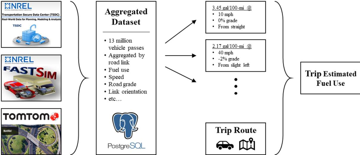
FIGURE 1 From left to right: the data pre-processing and powertrain simulation steps, the results of which are aggregated into a large data set from which an energy estimation look-up table for that particular vehicle model can be generated. Trip fuel use is estimated by combining the model results with a proposed trip route.
